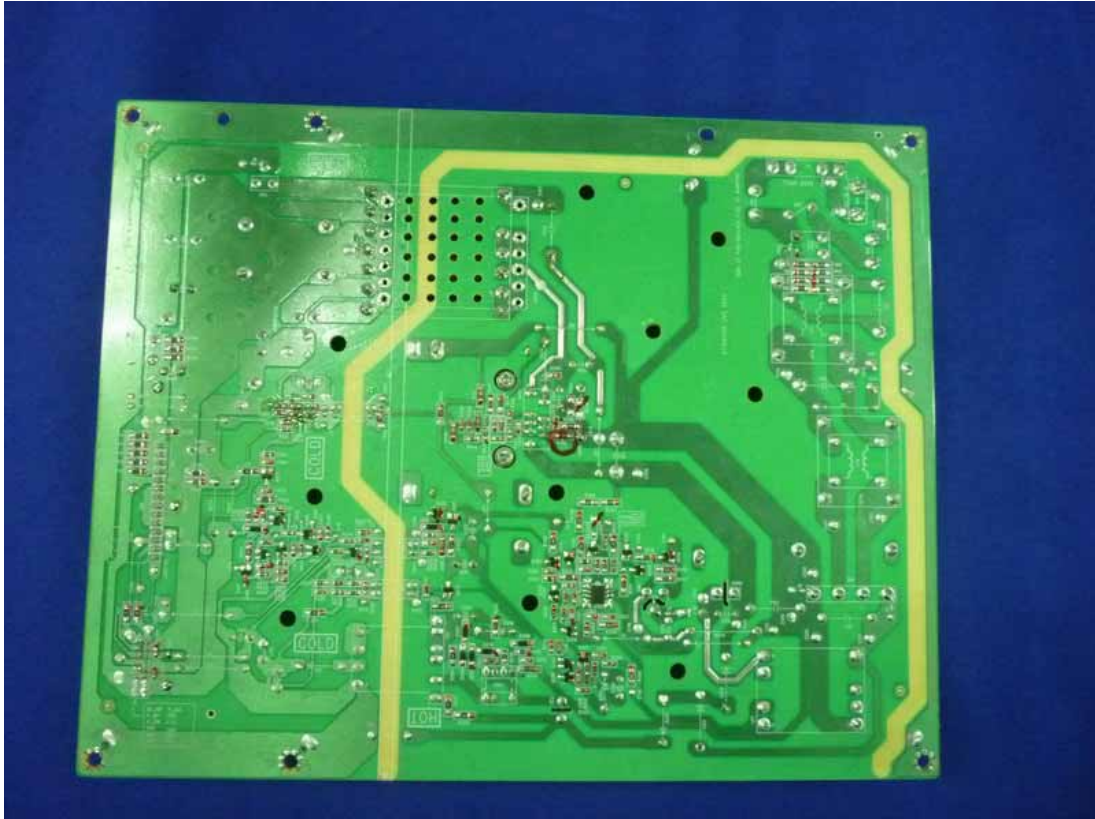
Figure 21 Backside of the Power Board
