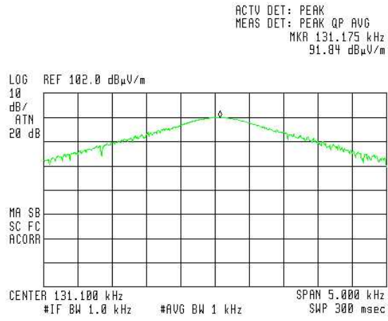
Figure 14. Field Strength of Fundamental, High
