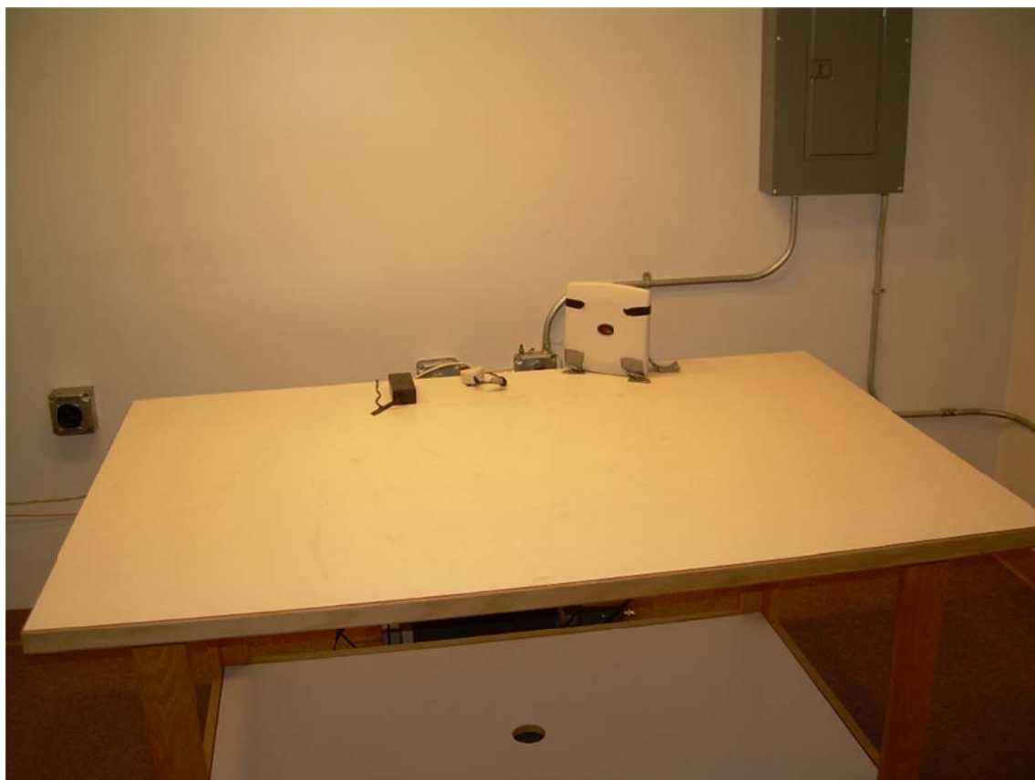
Front View Worst-Case Conducted Emissions Configuration
