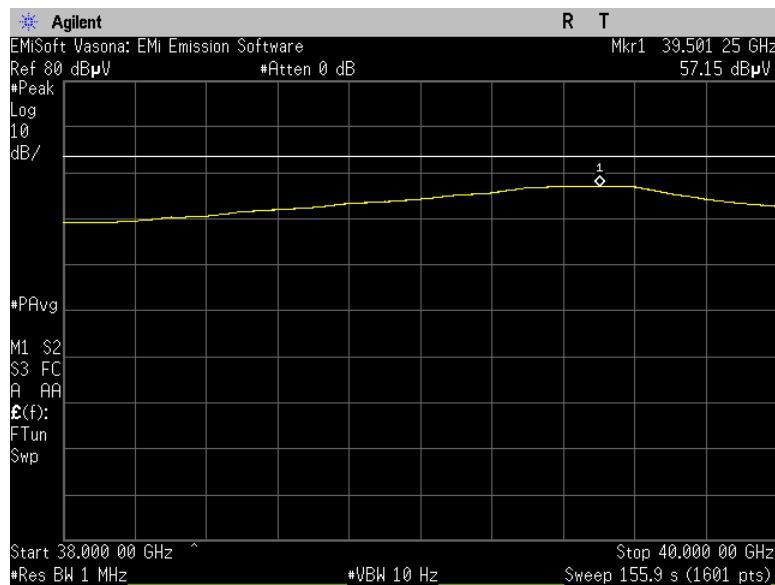
**Note:** The plot above shows reduced VBW for average measurements compared to average limit, thus the EUT complies with 38-40 GHz frequency range average limit requirement.
