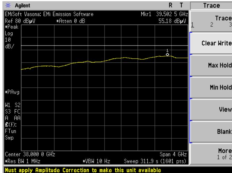
**Note:** The plot above shows reduced VBW for average measurements compared to average limit, thus the EUT complies with 36-40 GHz frequency range average limit requirement.
