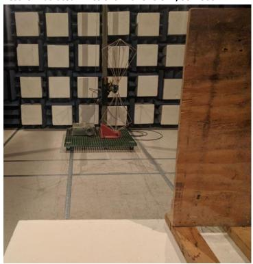
2. Test for Radiated Emissions with SAS-510-2, 300-1,000MHz
