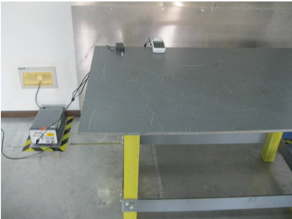
Conducted Emission Test Setup Front View
