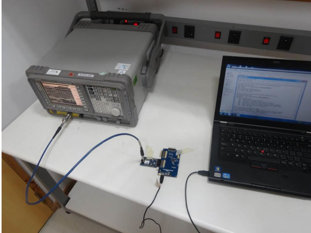
Conducted measurement Test setup
