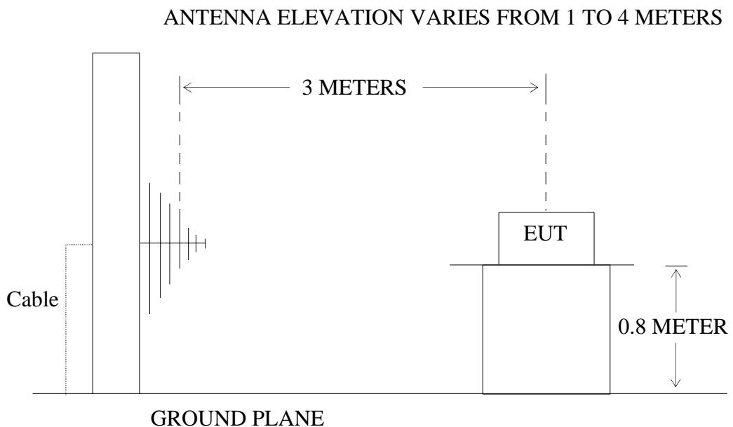
(EUT: Wireless Thermometer Hygrometer)
