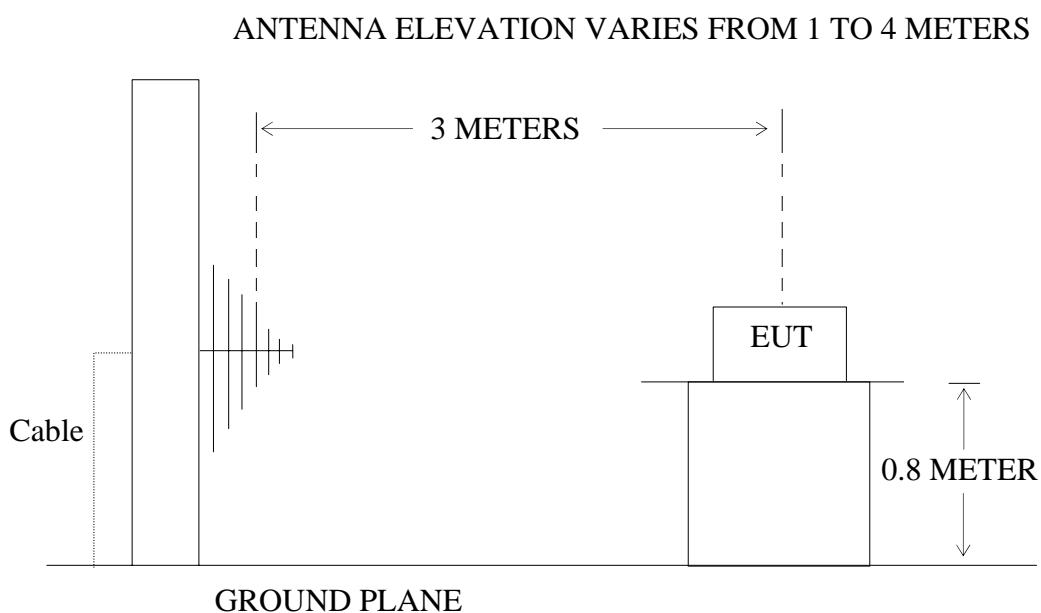
(EUT: Wireless Thermometer Hygrometer)
