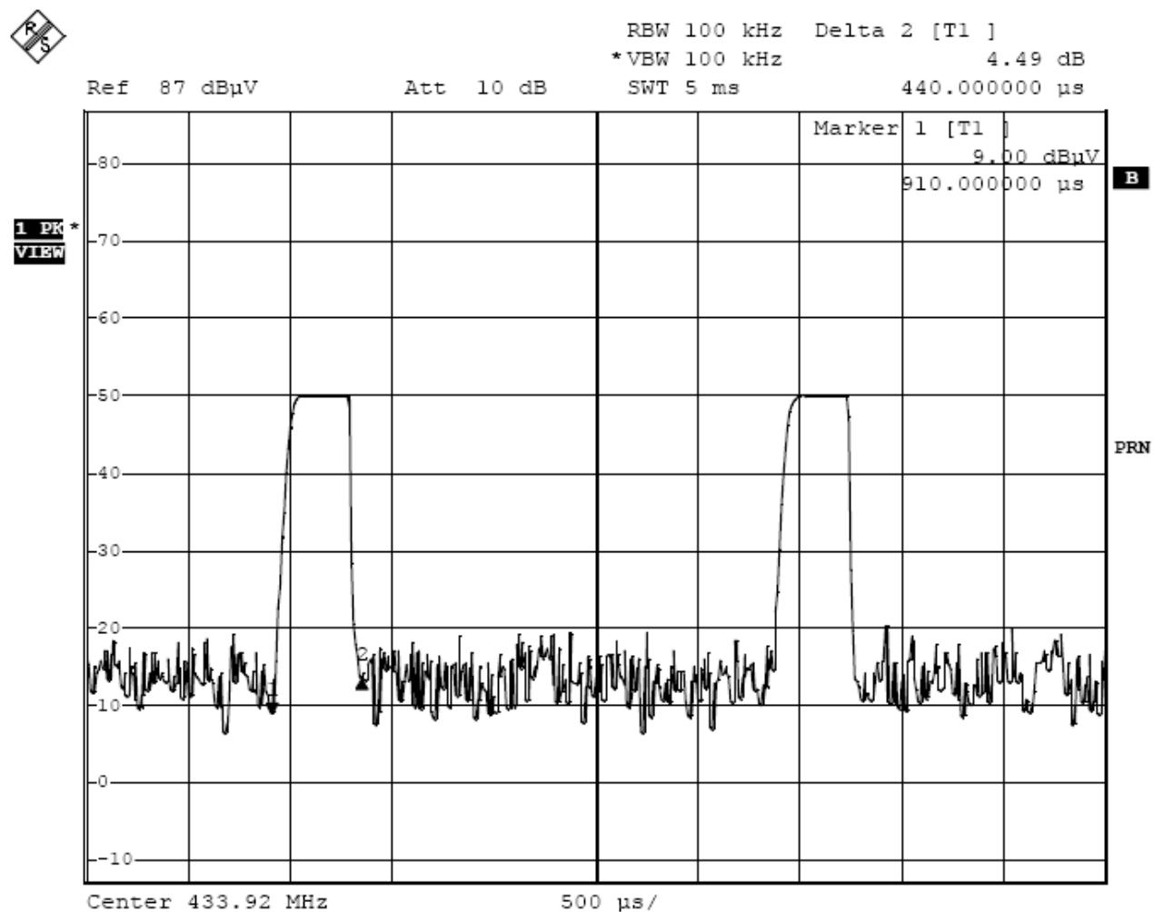
The graph shows the duration of 'on' signal. From marker 1 to marker 2, duration is 0.44ms.
