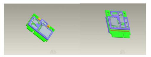
All components except the two antenna connectors are covered by EMC shields. All power and communication is routed through the edge connector of the card. The fastening holes in the upper corners are connected to ground.
