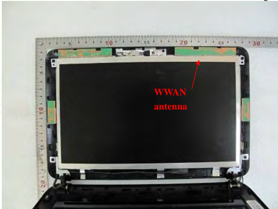
Fig.3 Antenna position of EUT
