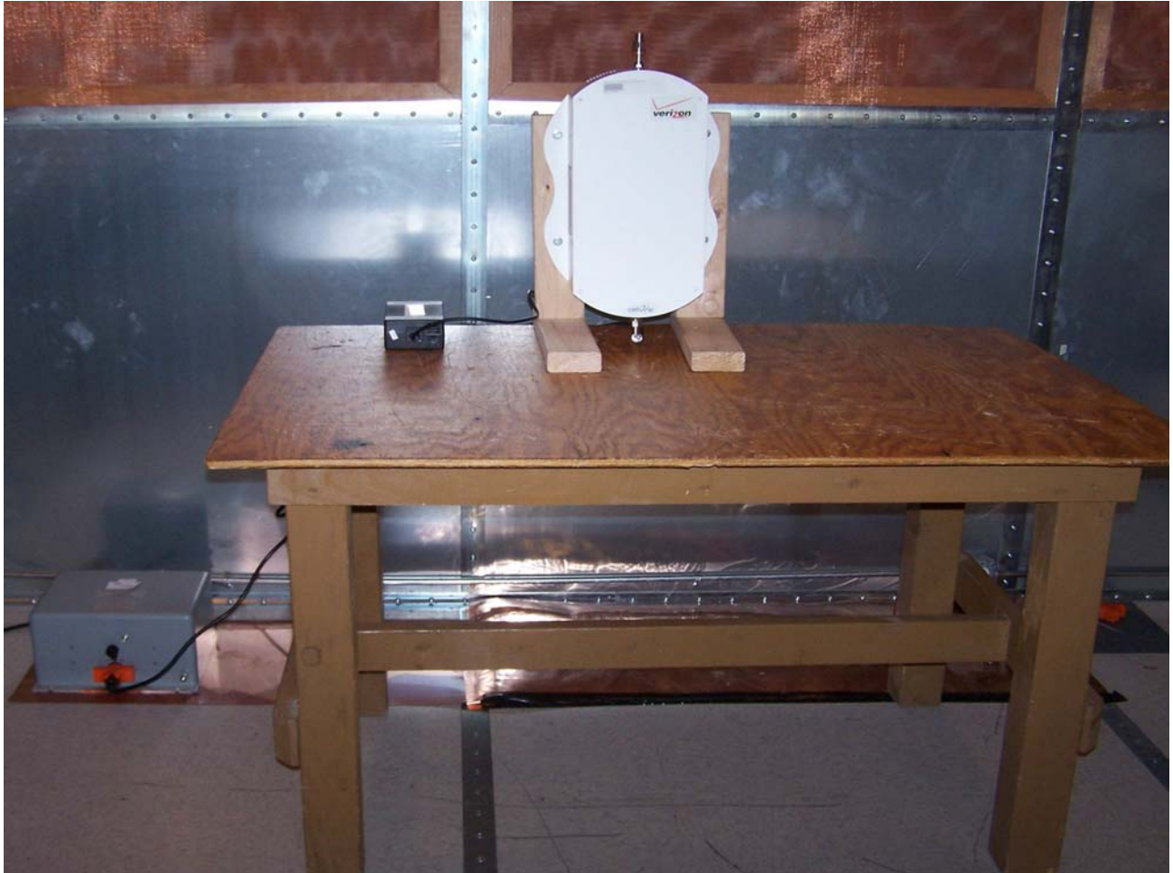
Photograph 2. Conducted Emissions Test Setup
