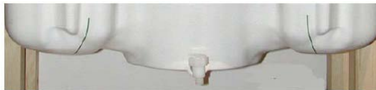
Figure 3.7 Sam Twin Phantom shell
