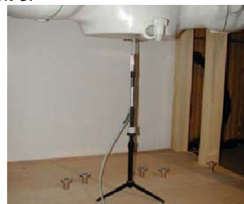
Figure 10.1 Dipole Verification Test Setup
