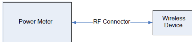
Figure 9.1 Power Measurement Setup
