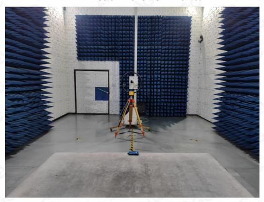
RADIATED EMISSION TEST SETUP BELOW 1GHz
