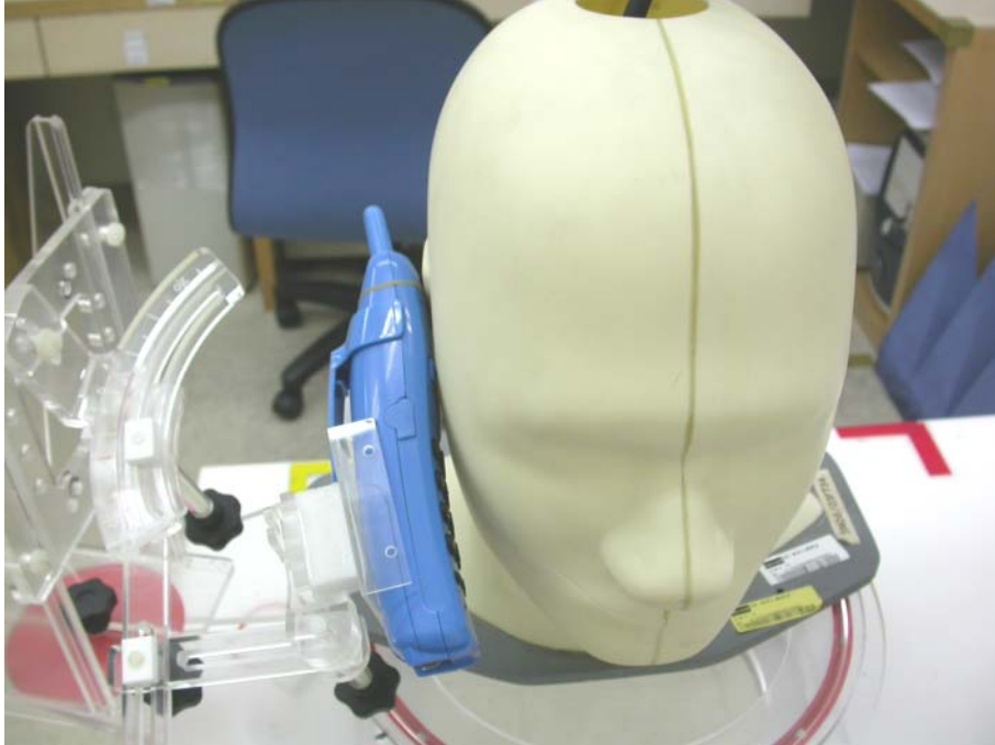
SAR Measurement Test Setup Cheek Position of Right Ear (with keypress)
