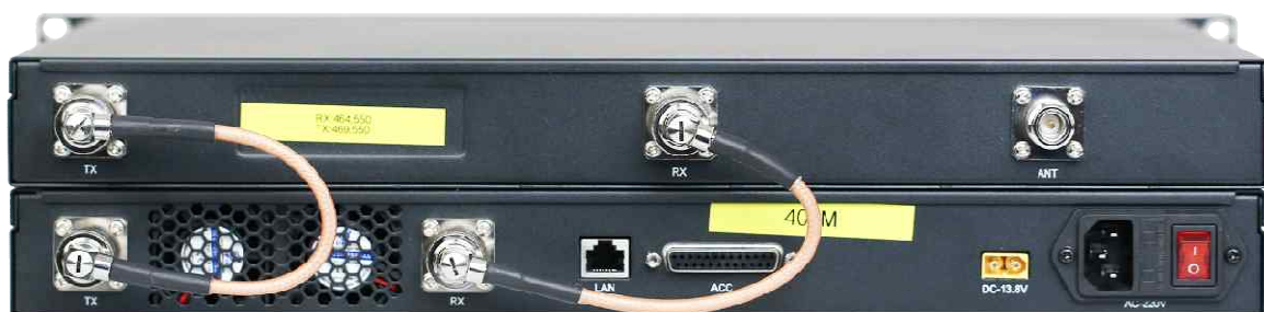
Figure 2-4) Duplex connection form with repeater
