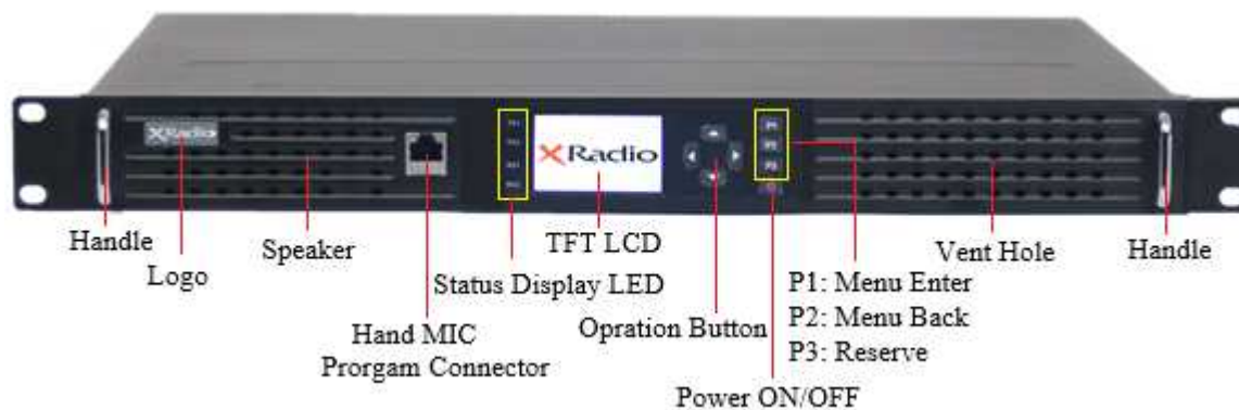
Figure 2-1) XR-R1100 Front Appearance Description
