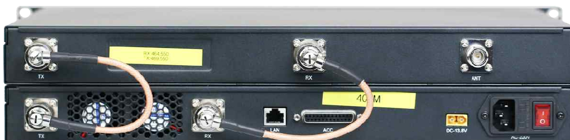
Figure 2-4) Duplex connection form with repeater
