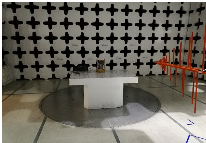
Radiated Emissions (>1GHz) - Front View
