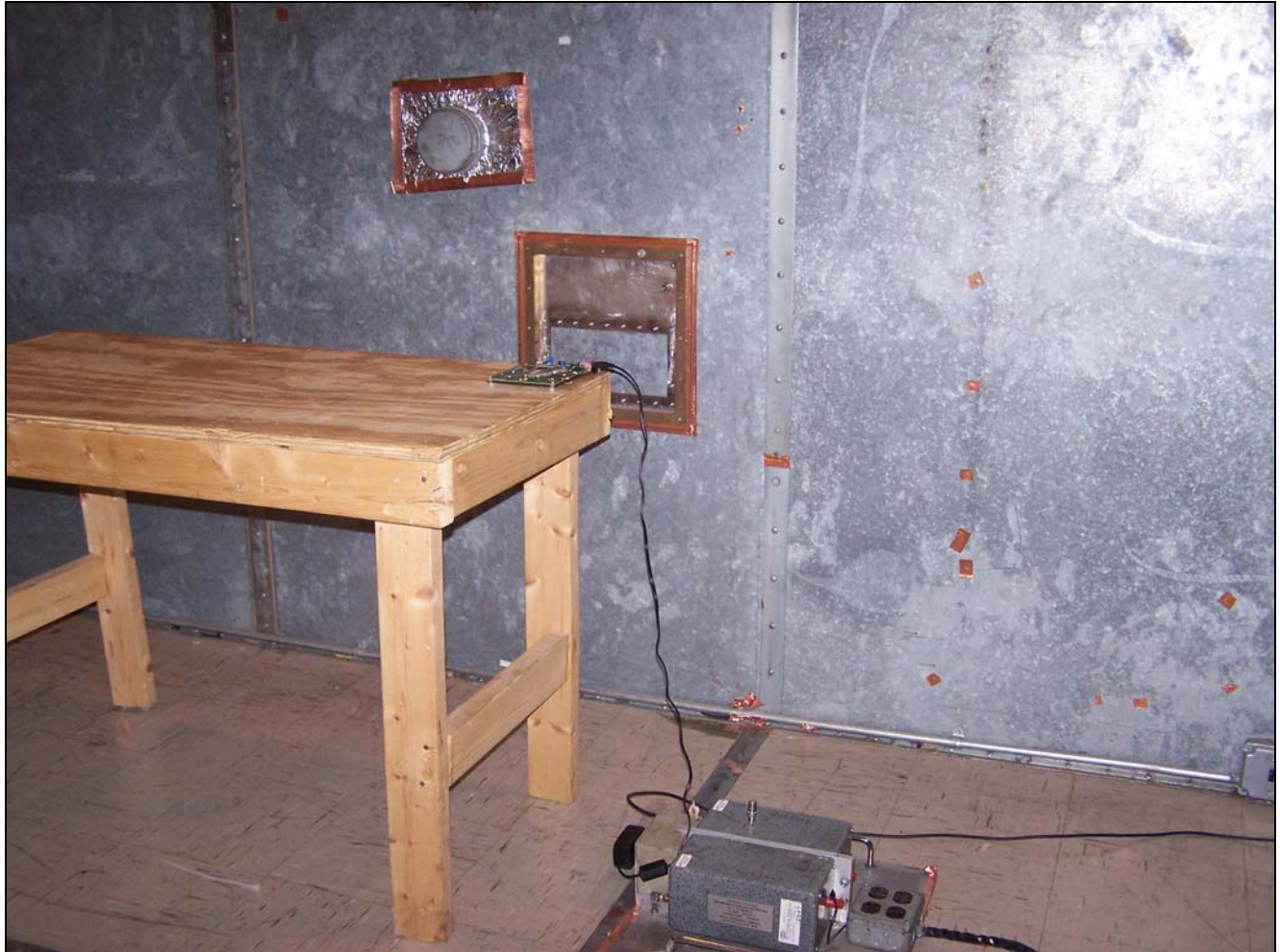
Photograph 2. Conducted Emissions, Test Setup
