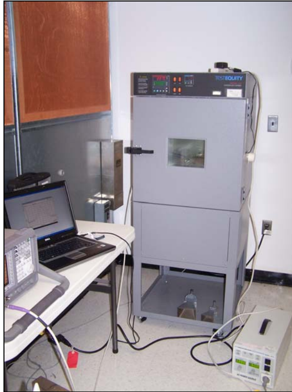
Photograph 6. Frequency Stability, Test Setup
