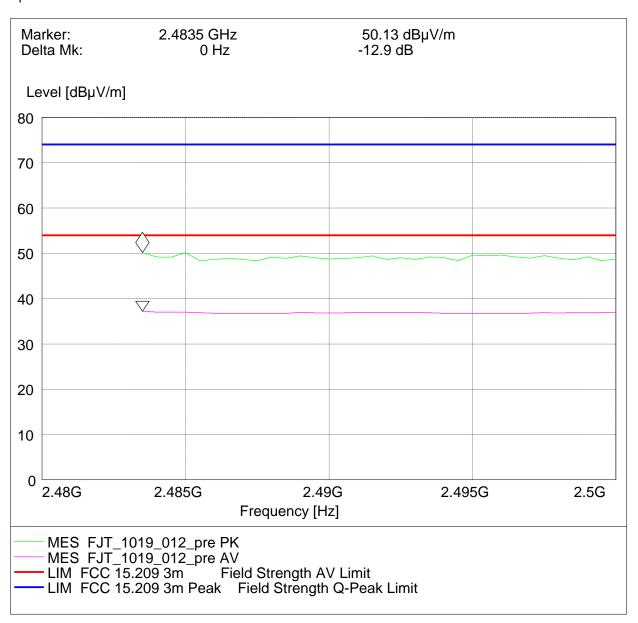
Radiated measurement (higher band edge)
