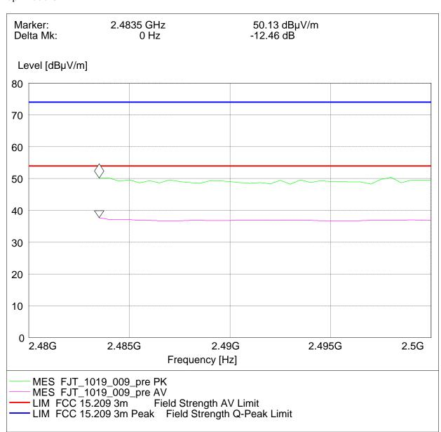
Radiated measurement (higher band edge)
