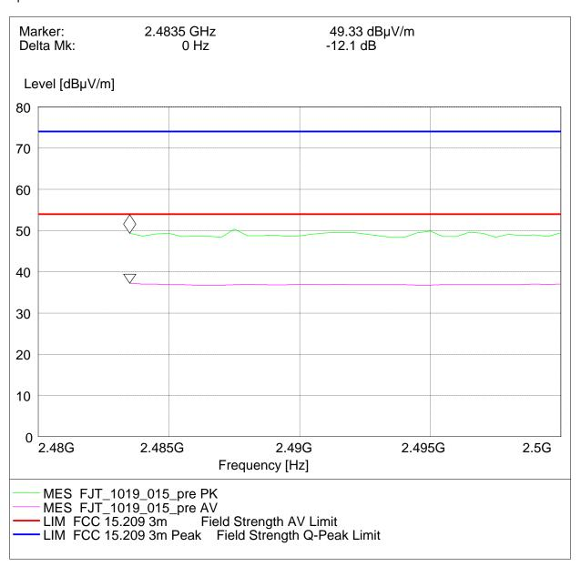
Radiated measurement (higher band edge)
