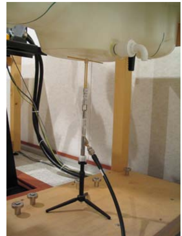
Photo of the dipole Antenna
