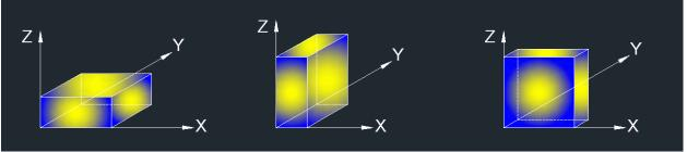
Remark 1: For all radiated test, EUT in each of three orthogonal axis emissions had been tested, but only the worst case (X axis) data recorded in the report.
