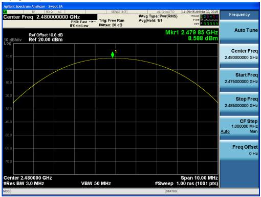
Test Plots (8DPSK) Peak Power (Low-CH)
