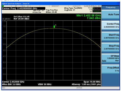
Test Plots (π/4DQPSK) Peak Power (Mid-CH)
