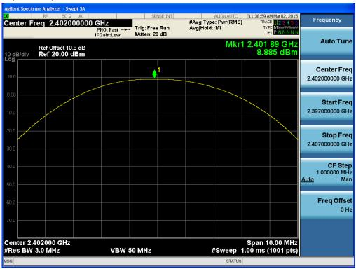
Test Plots (GFSK) Peak Power (Mid-CH)
