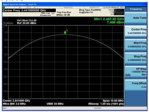
Test Plots (8DPSK) Peak Power (High-CH)
