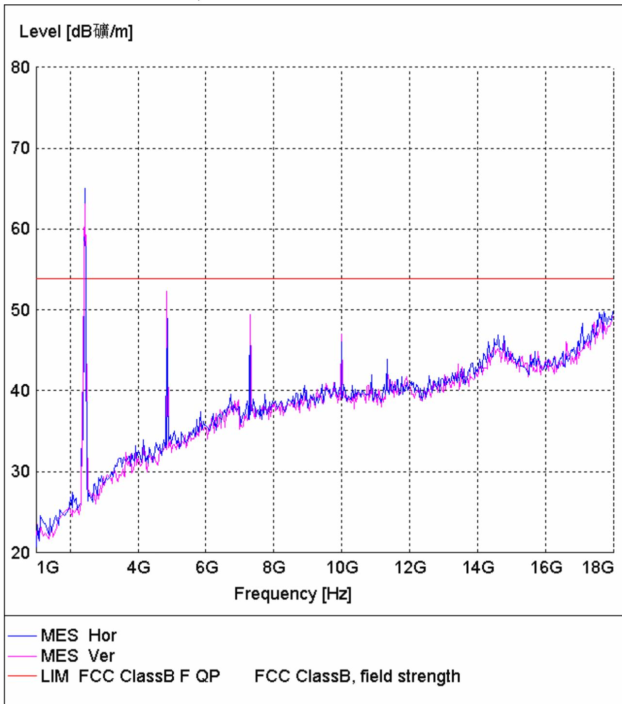
*Radiated Disturbance**EUT: 6 Channel model transmitters**M/N: FLYSKY001**Operating Condition: Transmitting below 1GHz**Test Specification: Vertical & Horizontal**Comment: DC 12V/Battery*
