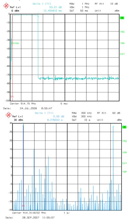
That gives a maximum of 1 transmissions in a period of 100 ms so the duel time correction factor for spurious measurement should be 20Log(12.4/100) = -18.1 dB.
