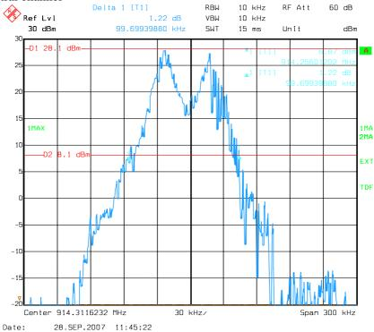
The 20dB bandwidth of each hopping channel is 100 kHz (less than 250 kHz)
