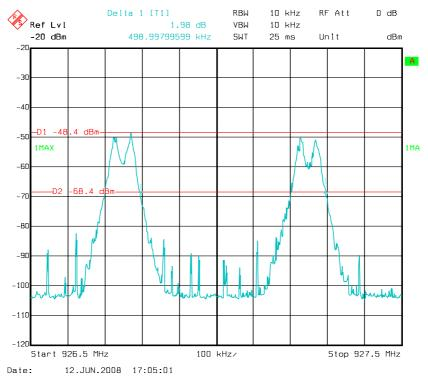
The channel separation is between 440kHz and 560 kHz (with an average at 500kHz) which is greater than the 20dB bandwidth.
