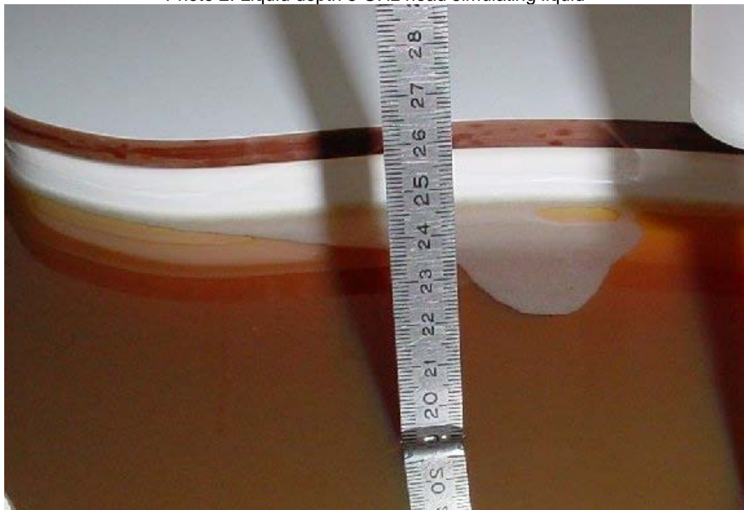
Photo 2: Liquid depth 5 GHz head simulating liquid
