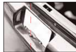
Fig.6 Camera Mounted on Bottom of License Plate
