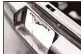
Fig.5 Camera Mounted on Top of License Plate
