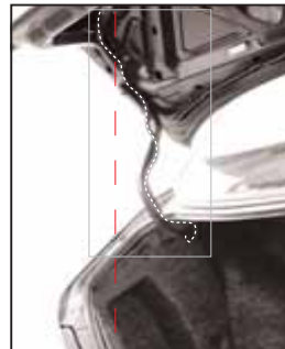
Fig.4 Camera Cable Routing on Hinge
