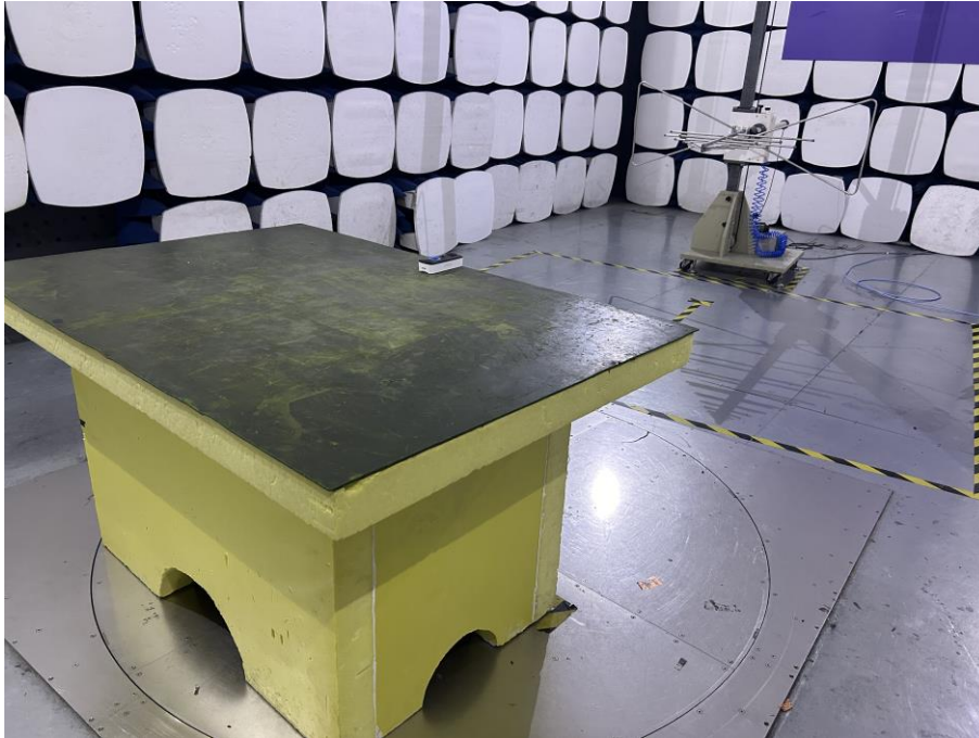
Spurious Emission Test Setup (Below 1GHz)
