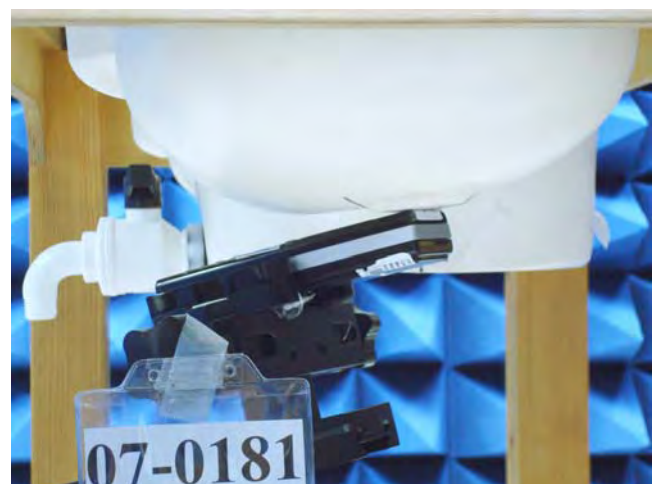
Figure 17. Left Head SAR Test Setup (Tilted)
