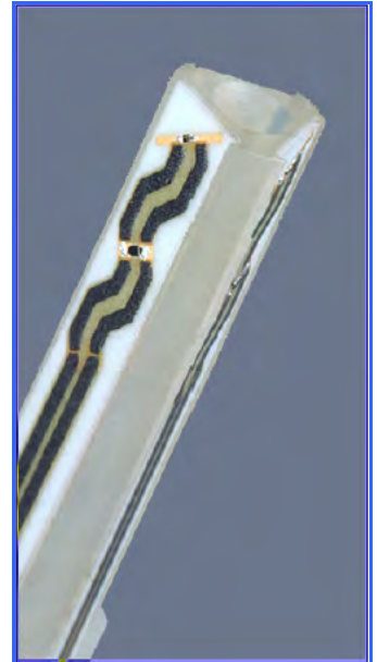
Figure 7. ET3DV6 E-field Probe
