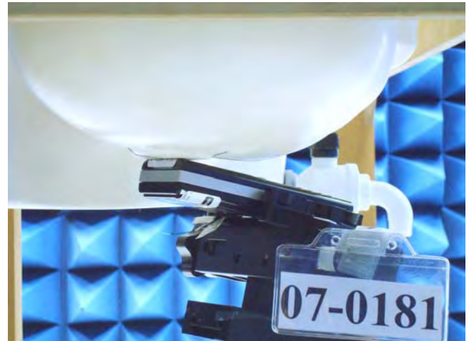
Figure 15. Right Head SAR Test Setup (Tilted)
