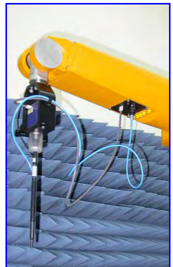
Figure 8. Probe setup on robot
