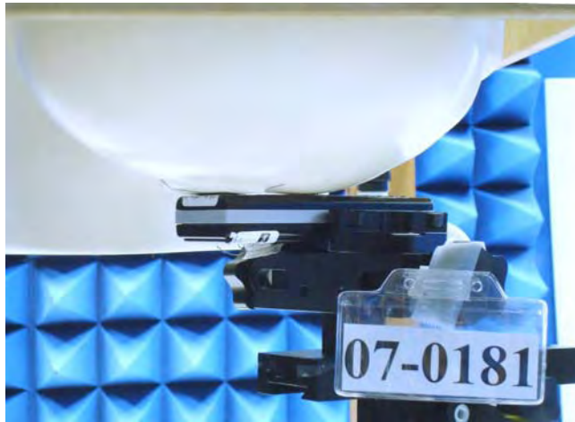
Figure 14. Right Head SAR Test Setup (Cheek)
