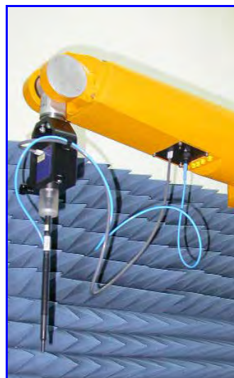
Figure 4. Probe setup on robot
