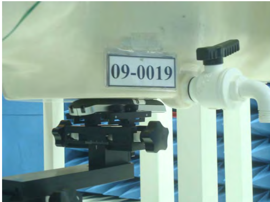
Figure 18. Body SAR Test Setup _ Back to Phantom 2mm separation
