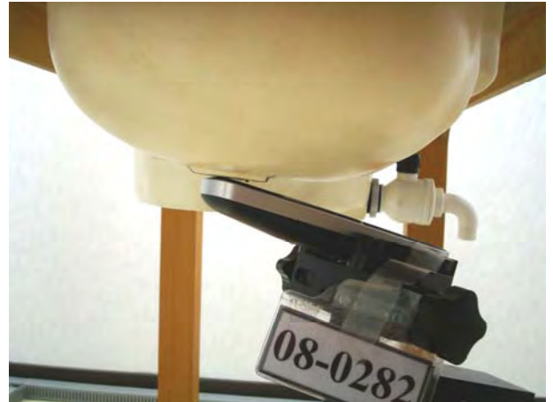
Figure 14. Right Head SAR Test Setup (Tilted)
