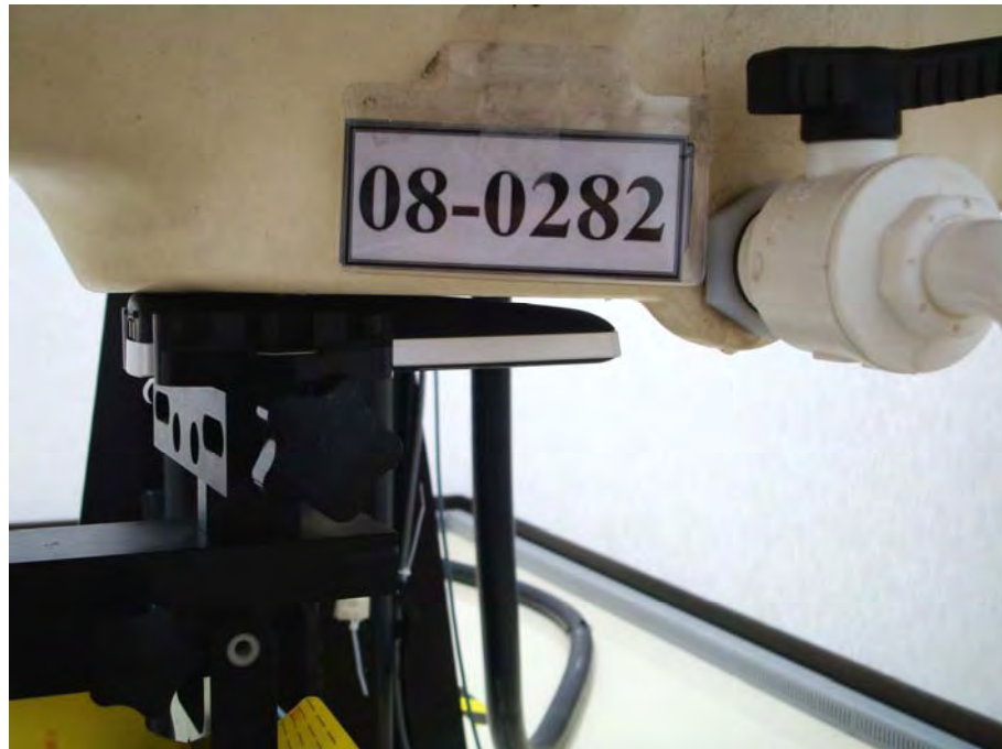
Figure 17. Body SAR Test Setup _ Back to Phantom 2mm separation
