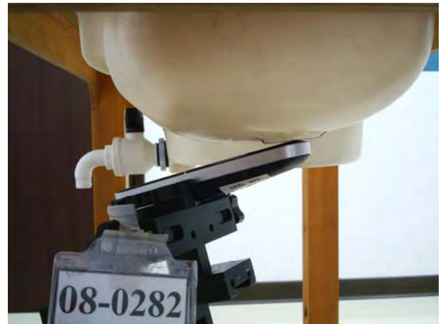
Figure 16. Left Head SAR Test Setup (Tilted)
