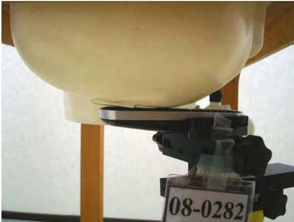
Figure 13. Right Head SAR Test Setup (Cheek)
