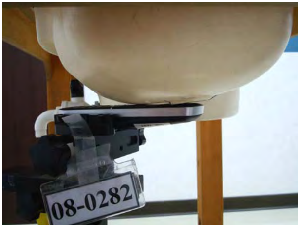
Figure 15. Left Head SAR Test Setup (Cheek)
