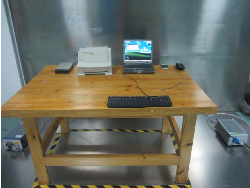
Conducted Emissions - Front View (USB Downloading)
