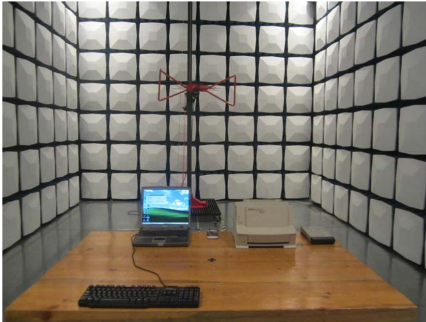
Radiated Emissions –Front View (Below 1GHz) (USB Downloading)
