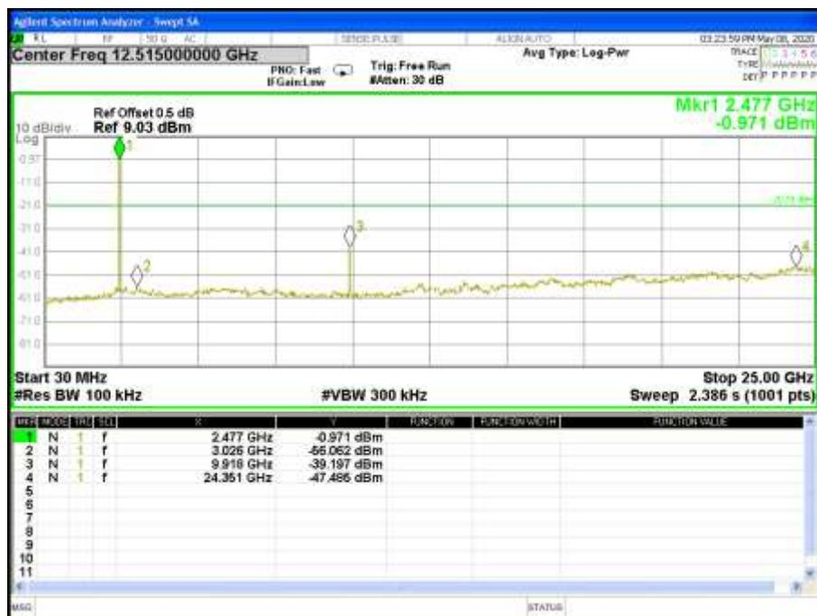
For Band edge(it's also the reference level for conducted spurious emission)
