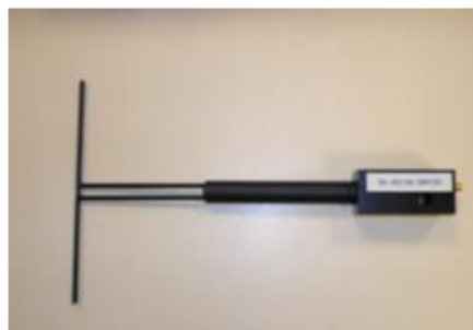
Figure 1 – Satimo COMOSAR Validation Dipole
