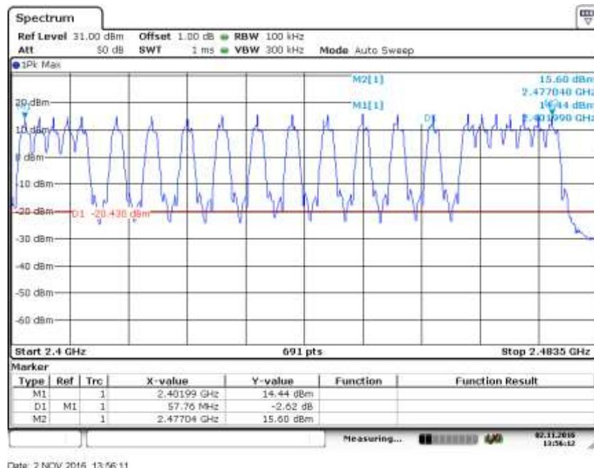
Remark: The product will only use 22 Channels (from Channel 1 to Channel 22) under normal operating condition. The last one Channel (Channel 23) is only used in matching mode.
