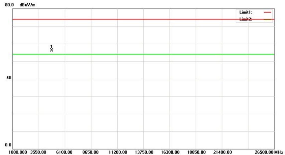
Figure 11 – Radiated emission data graph (Vertical polarization, 1GHz-26GHz) For Baby Unit
