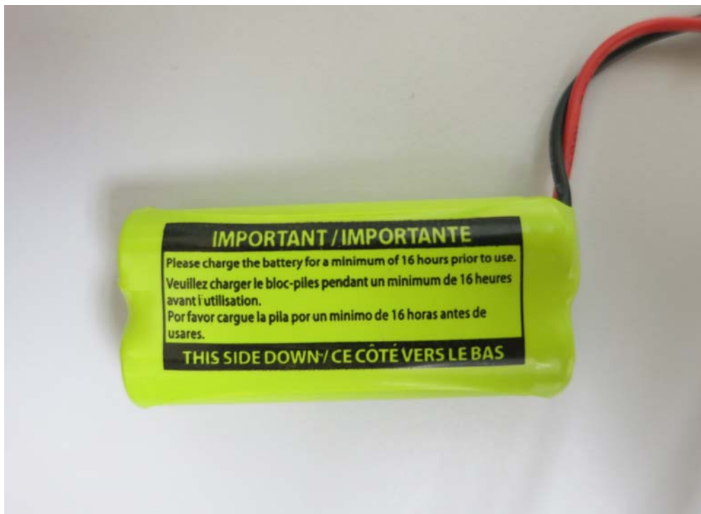
Figure 6 – 2.4V 400mAh Ni-MH Corun rechargeable battery back view
