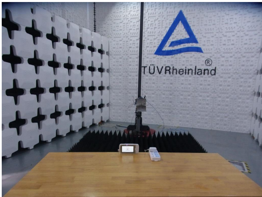
Photograph 5: Set-up for Radiated Emission, Above 1GHz
