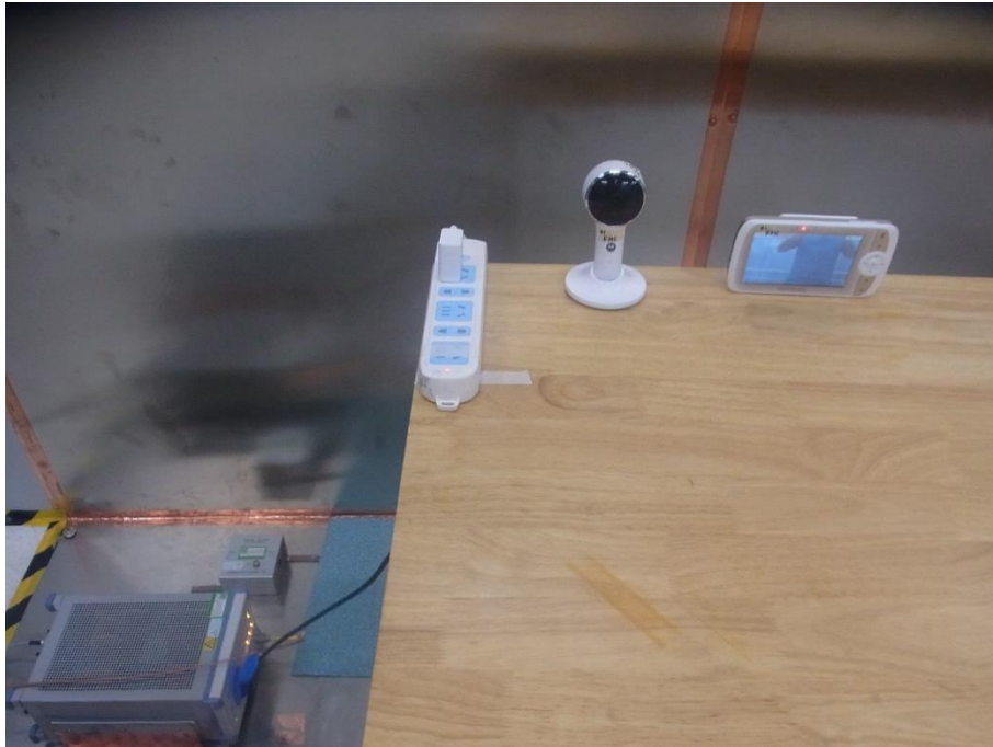
Photograph 3: Set-up for Conducted Emission on AC Mains
