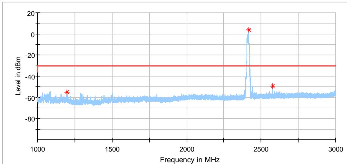
**Radiated emission data graph (Horizontal polarization, 1GHz-3GHz)**
