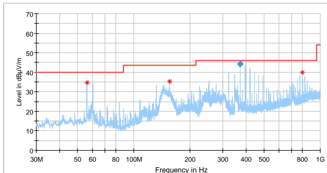
**Radiated emission data graph (Vertical polarization, 30MHz-1GHz)**
