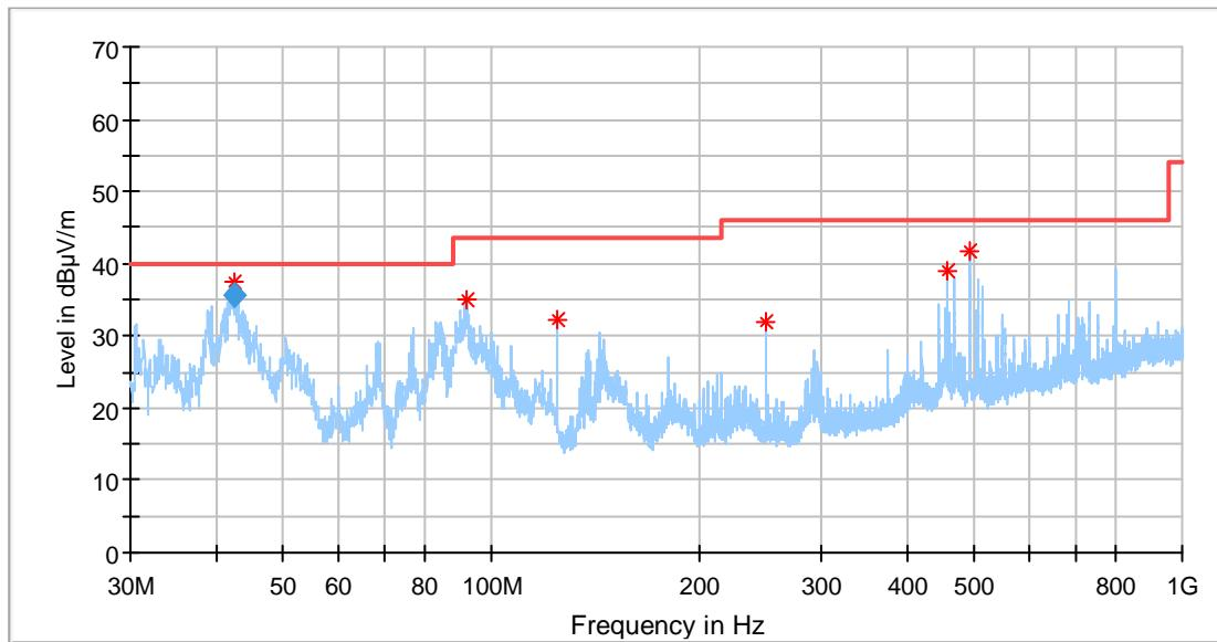
**Radiated emission data graph (Horizontal polarization, 30MHz-1GHz)**
