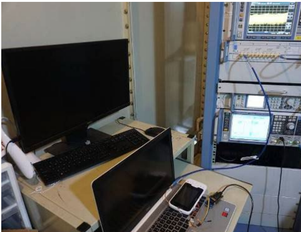
Conducted RF Output Power Test Setup
