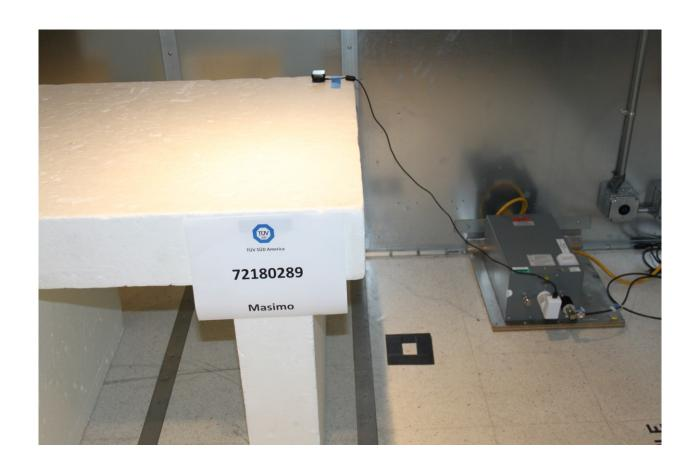
**AC Conducted Emissions Test Setup**
