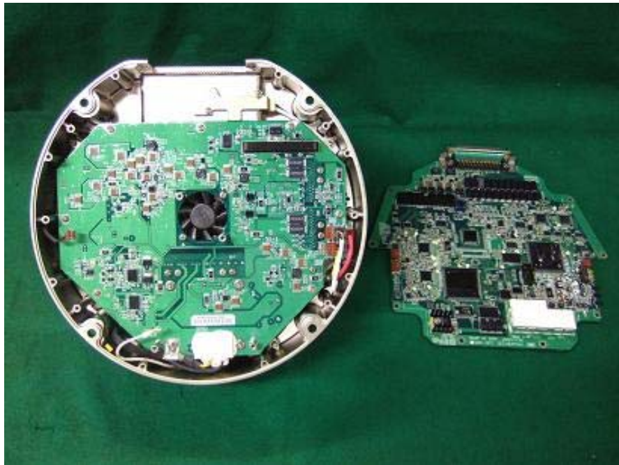
MOD/PS Bottom view and RCV/CONT Top view (RCV/CONT removed)
