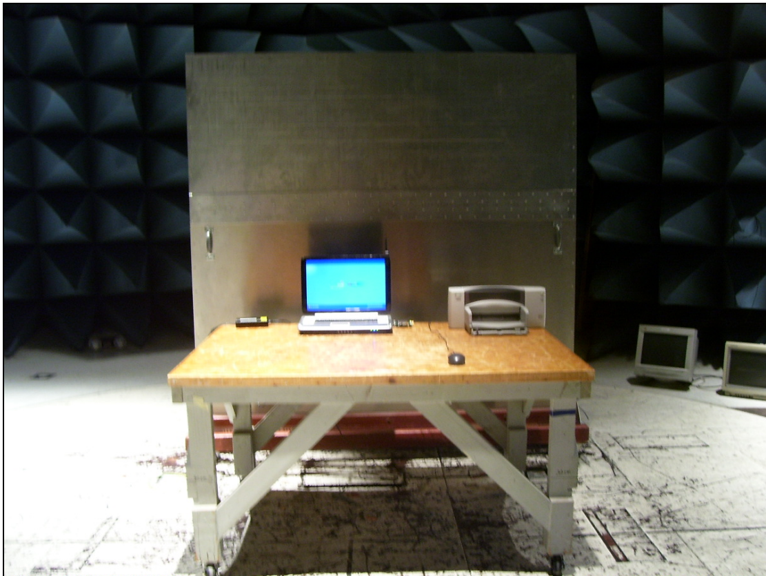
Photograph 2. Conducted Emissions Test Setup – Front View
