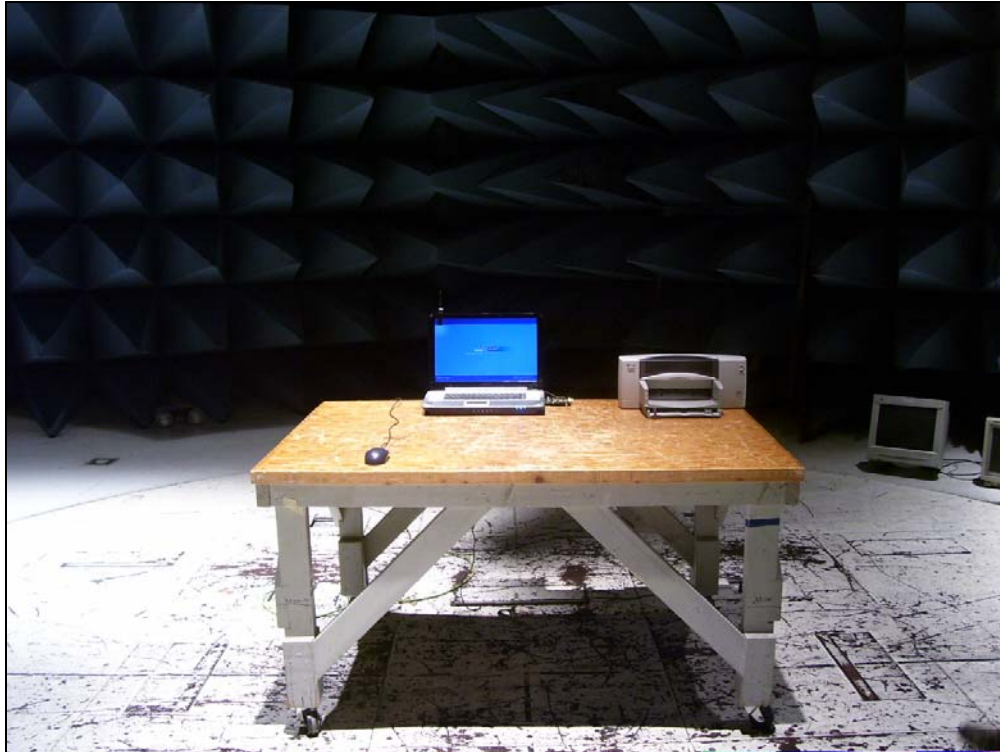
Photograph 4. Radiated Emission Test Setup 30 MHz - 1 GHz
