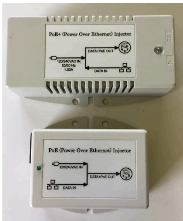
The approved use of any Rajant-supplied AC-powered mid-span Power-over-Ethernet (PoE) power supply (see illustration) is limited to indoor, environmentally-sheltered, non-damp locations that are isolated from shock and vibration. These power supplies are not sealed for dust or water ingress and are not intended to operate in an environment with condensing humidity. The construction of these power supplies is not ruggedized for exposure to mechanical shock or vibration.
