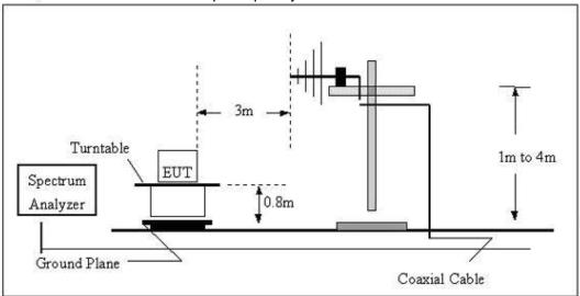
2. Radiated Emission Test Set-Up Frequency Above 1GHz
