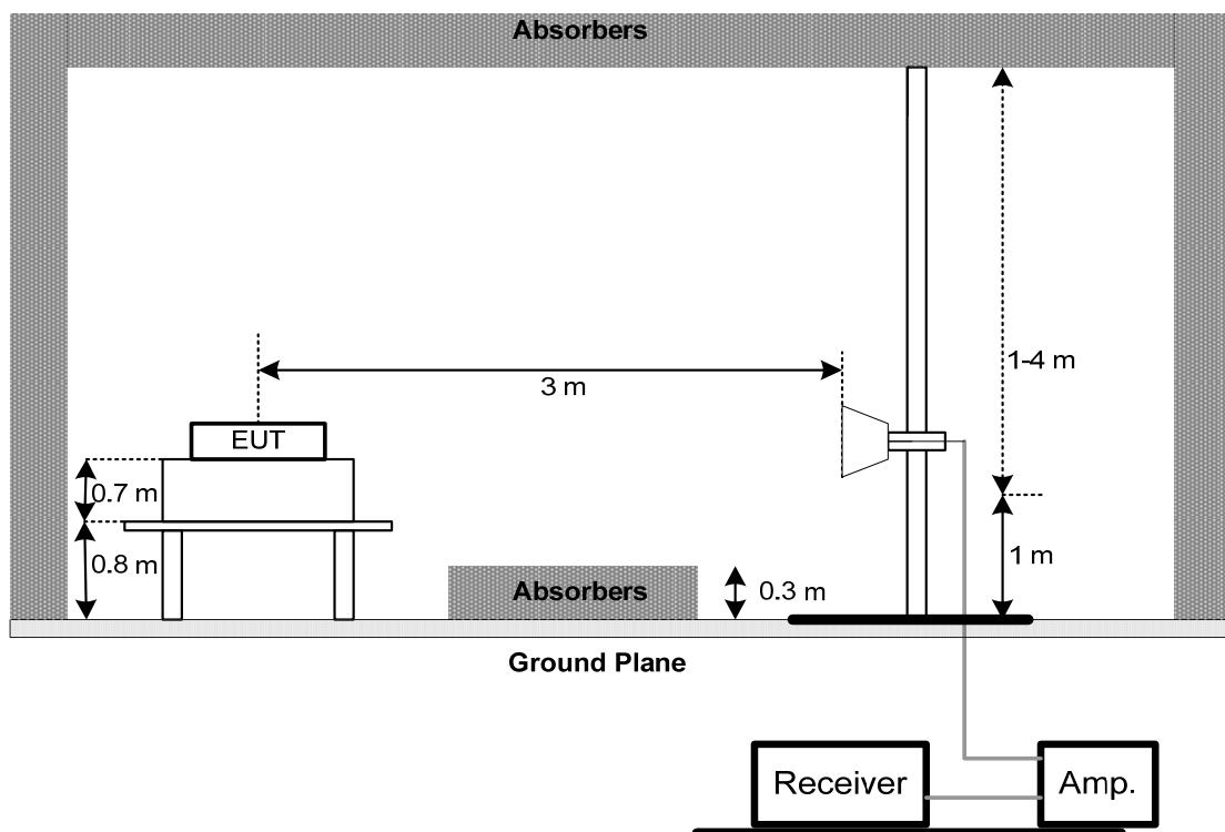
(C) For Radiated Emissions Below 30MHz
