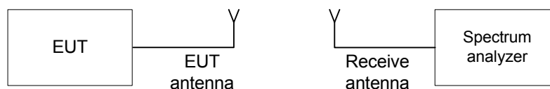
Figure 7.7.1 Band edge emission test setup
