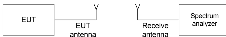
Figure 7.4.1 Carrier frequency separation test setup
