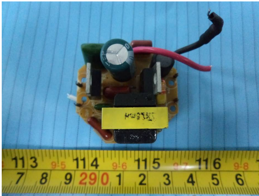
EUT – Main Board Top View
