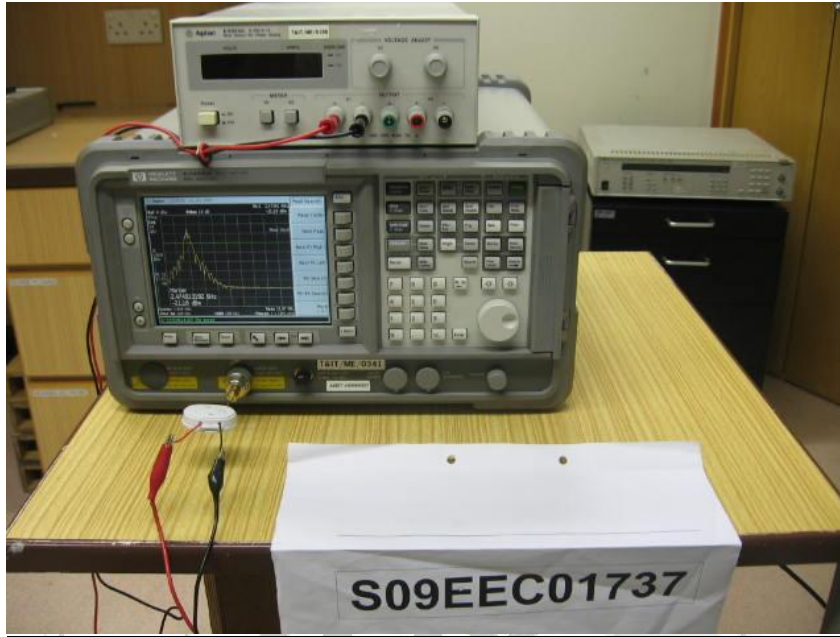
Spectrum Bandwidth (6dB Bandwidth Measurement) Test Setup
