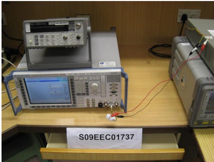
Maximum Peak Power Test Setup
